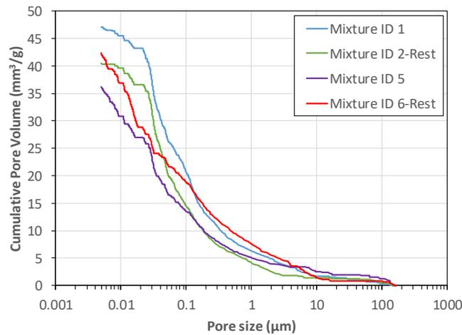
Fig. 3. Cumulative pore volume distribution for Mixture IDs 1, 2-Rest, 5 and 6-Rest
