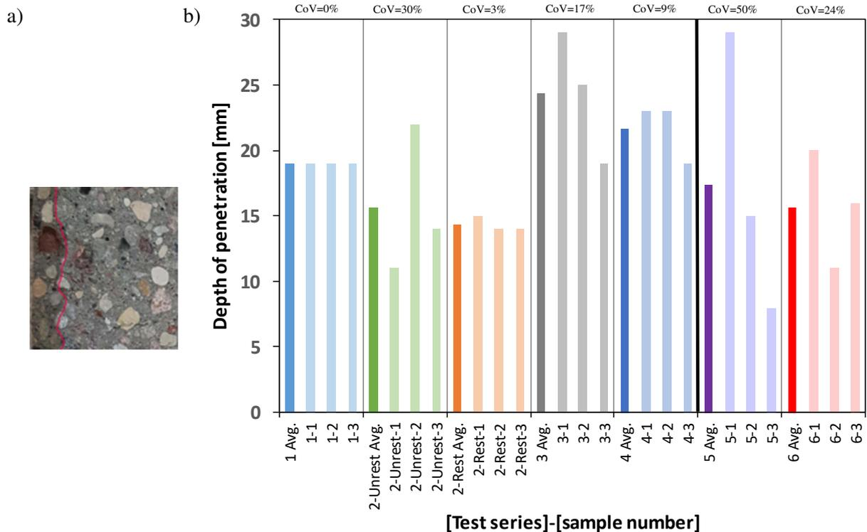
**Fig. 2. Image of clear colour difference, used to measure the maximum water penetration depth and (a) measured average (dark colour) and individual (pale colours) water penetration depths for the various Mixture IDs (b)**
