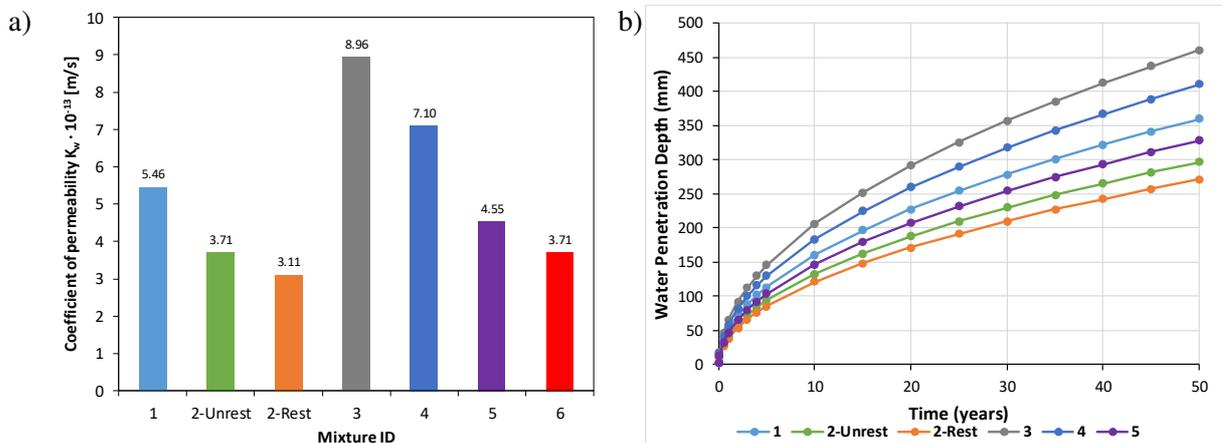
Fig. 5. Computed coefficient of permeability, per equation (1), for the indicated Mixture IDs (a) and estimated water penetration depths for the indicated Mixture IDs (b)
