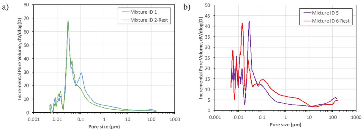
Fig. 4. Pore size distribution for the 0.55 w/c ratio mixture IDs 1 and 2-Rest (a) and the 0.40 w/c ratio mixture IDs 5 and 6-Rest (b)
